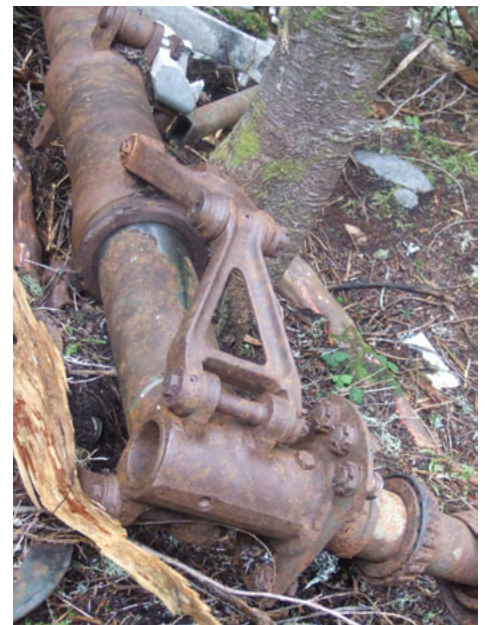
This landing gear is among the few pieces to have rusted. It's steel, of course; most of the remaining wreckage is aluminum.
